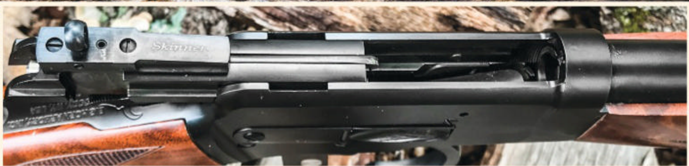
The M89's open-top design ejects fired cartridges straight up, and the bolt reciprocates on rails machined into the inner walls of the receiver. Big Horn Armory mounts a Skinner aperture sight.
